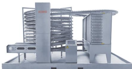
◆ No rotating cage, making the internal space easier to clean and inspect.
